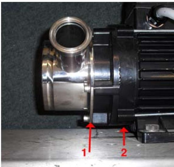
Fig. 4. Leak at Arrow 1 is minor and easily resolved by snugging up the pumphead (or changing a large oring). Leak at Arrow 2 is due to corroded seals and must be resolved promptly.
