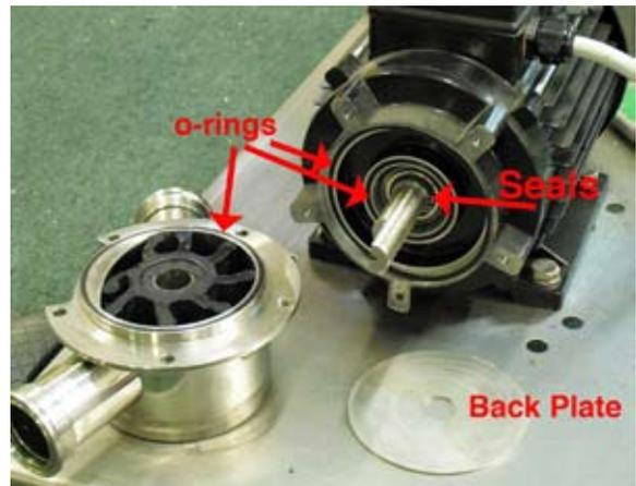
Fig. 3. Remove, clean, and lubricate pumphead regularly.
