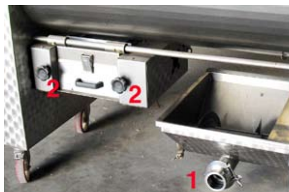
Fig. 2. "1" is outlet (3" TC) for must pump. There is an identical outlet on other side. Choose whichever side is most convenient. "2" are roller adjustment knobs. In this photo, the unit operates as destemmer only. The rollers must be slid to the right to operate as a destemmer/crusher.
