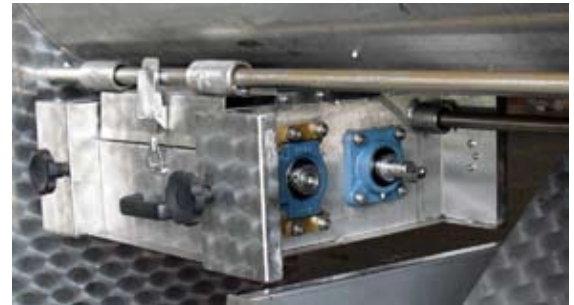
Fig. 4. Roller bearings exposed when side panels are removed. Remove side panels to lubricate. Do NOT pressure wash bearings.
