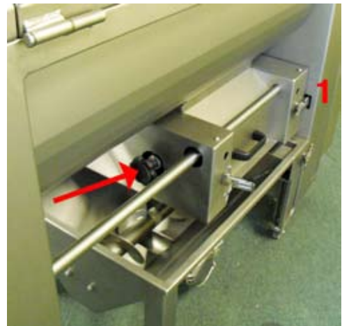
Fig. 3. Turn black knob to disconnect rollers.
