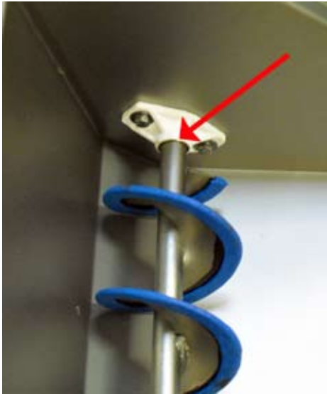
Fig. 7. Lubricate the bushing in hopper annually.
