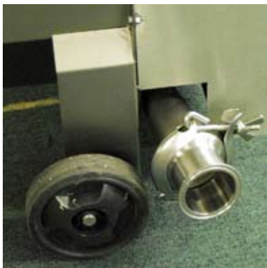
Fig. 2. Outlet for built-in must pump. 2.5" TC. Be certain that liquid is drained from the pump after each use and cleaning.
