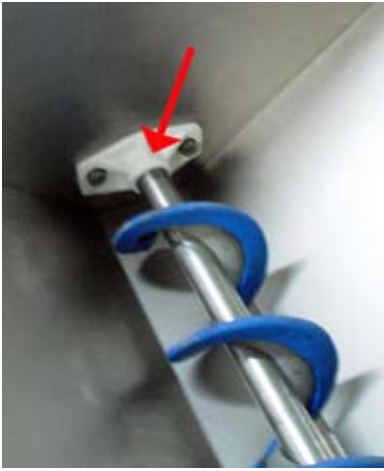
Fig. 5. Auger/bushing lubrication point.
