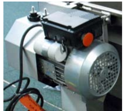
Fig. 1. motor and power switch.
