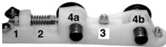
Fig. 8. Rubber rollers are mounted in spring-loaded bracket on one end. This spring system protects the rollers from damage if a large item (stone for example) is in the fruit.
