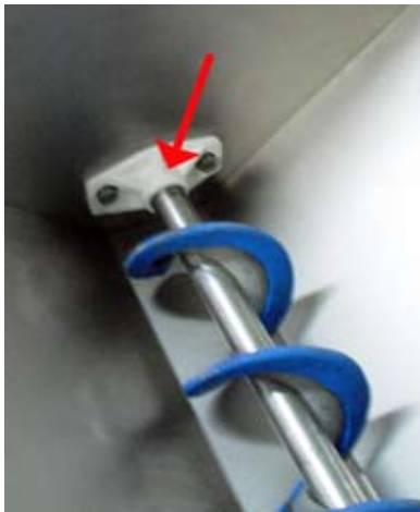
Fig. 5. Auger/bushing lubrication point.
