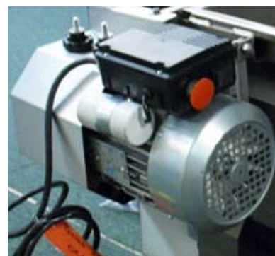
Fig. 1. motor and power switch.
