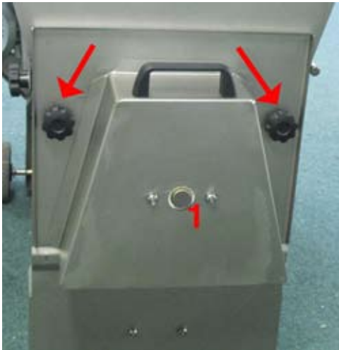
Fig. 3. Remove the two black knobs and pull out the destemming basket. [“1” is a destemming shaft/bushing lubrication point.]
