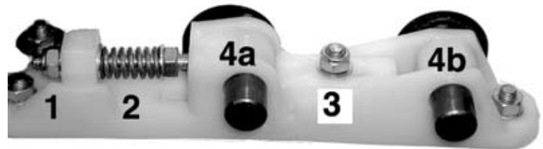
Fig. 7. Rubber rollers are mounted in spring-loaded brackets. This spring system protects the rollers from damage if a large item (stone for example) is in the fruit.
