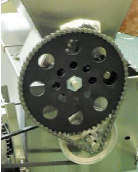
Fig. 6. Remove end cover annually and lubricate chains and gears. To not grease the V-belts. Do not wash down these components.
