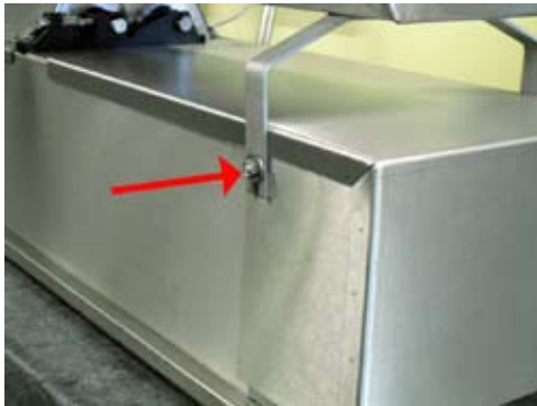
Fig. 2. Loosen the nut indicated by the red arrow (and the nut on other side). Then slide the cover off.
