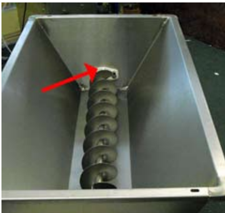
Fig. 5. Lubricate bushing indicated by the arrow annually. See also "1" in Fig. 2.
