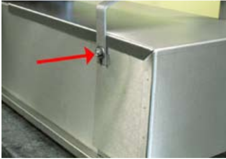
Fig. 2. Loosen the nut indicated by the red arrow (and the nut on other side). Then slide the cover off.
