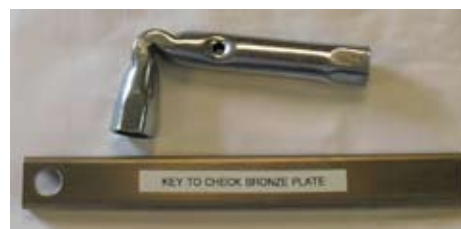
Fig. 4. Tools. The top wrench is used to open/close the pumphead. The lower is the “key wrench” used to access the bronze plate.
