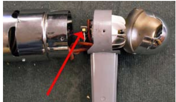
Figure 2. Arrow indicates location of a carbon brush.
