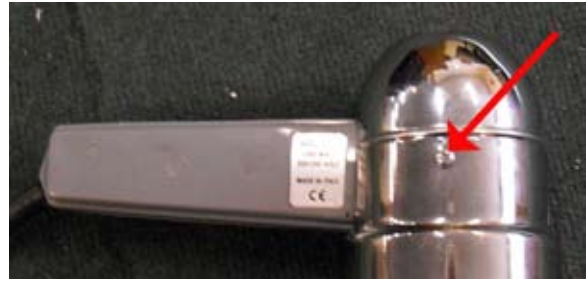
Figure 1. Remove this screw and the screw on opposite side.
