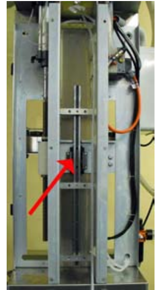
Figure 6. Back of unit with cover removed. Lubricate slide and rails annually.
