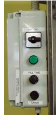
Figure 5. OFF/On switch at top with green indicator light below it. Fill Time adjustment. DRAIN button used only if product line is disconnected.
