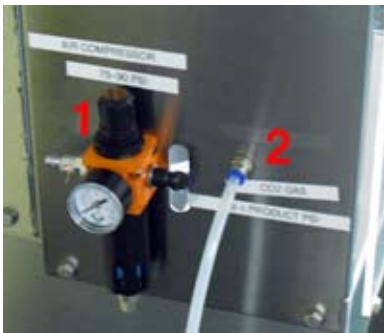
Figure 3. Attach air hose. Set your air compressor set to >90 psi. Adjust regulator (1) to 5-6 bar (75-90 psi). Attach CO 2 line to (2). CO 2 pressure must be less than product tank pressure. Max pressure of CO 2 line is 60 psi.
