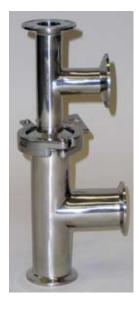
1" and 1.5" TriClamp use the same clamp. The 'ferrule' is the same. The difference is the pipe diameter. To demonstrate, a 1" Tee is attached directly to a 1.5" Tee.
