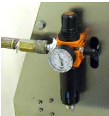
Fig. 5. Air line connected to regulator. Set air compressor pressure >80 psi. Set corker regulator to 70-80 psi.
