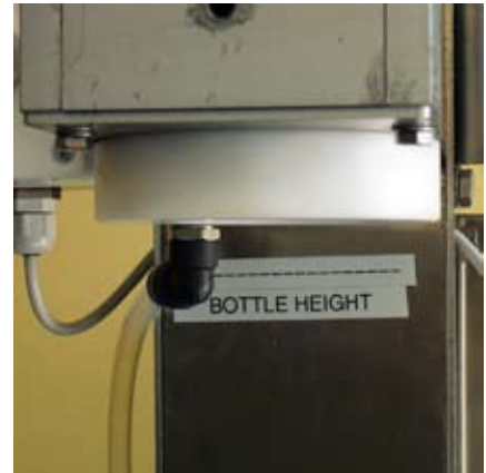
Fig. 1. Bottle Height---Top of bottle MUST be at this height or slightly higher.
