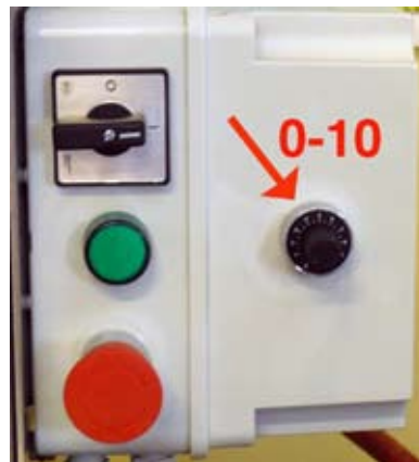
Fig. 6. Dial to precisely determine the length of cork above the top of bottle neck.
