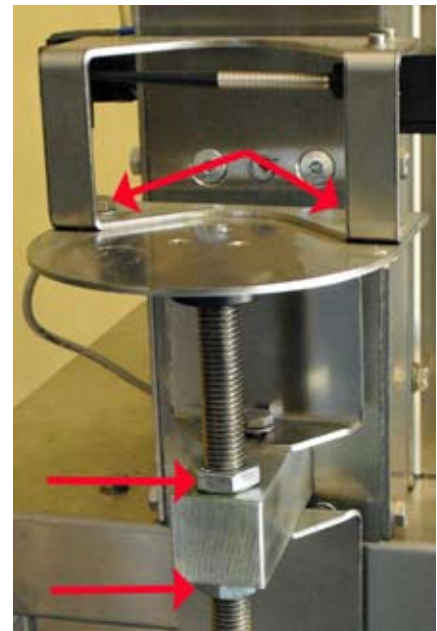
Fig. 2. Raise or lower bottle stand. Adjust Back Support to match Bottle Diameter.
