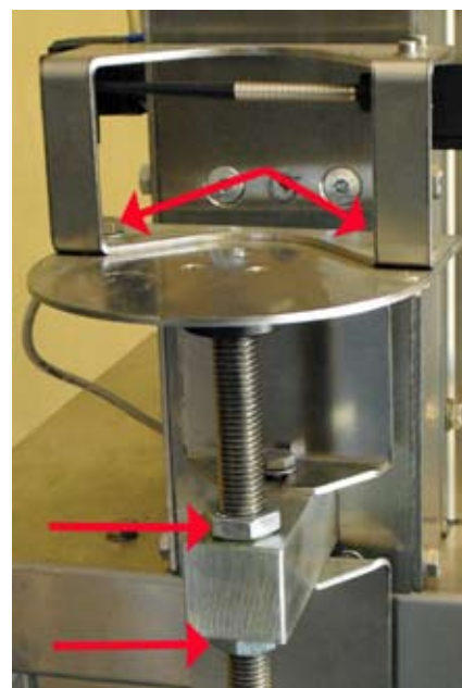
Fig. 2. Raise or lower bottle stand. Adjust Back Support to match Bottle Diameter.
