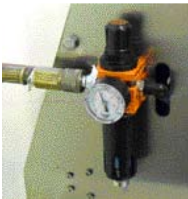
Fig. 4. Air line connected to regulator. Set air compressor pressure >80 psi. Set corker regulator to 70-80 psi.
