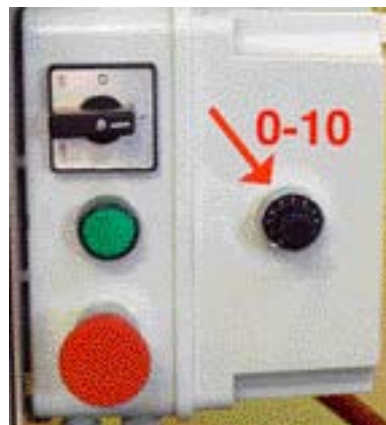
Fig. 5. Dial to precisely determine the length of cork above the top of bottle neck.
