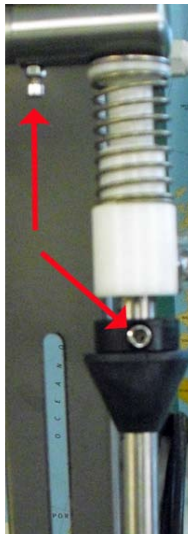
Figure 2. Do NOT overtighten these bolts.
