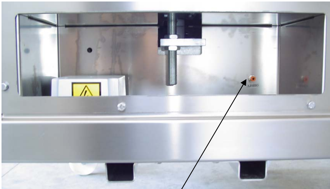
Connection for azote-feeding pipe
