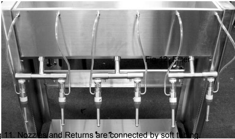
Fig 11. Nozzles and Returns are connected by soft tubing
